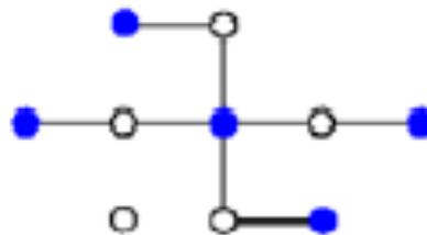
A vertex cover of size 5 obtained by the greedy algorithm.
